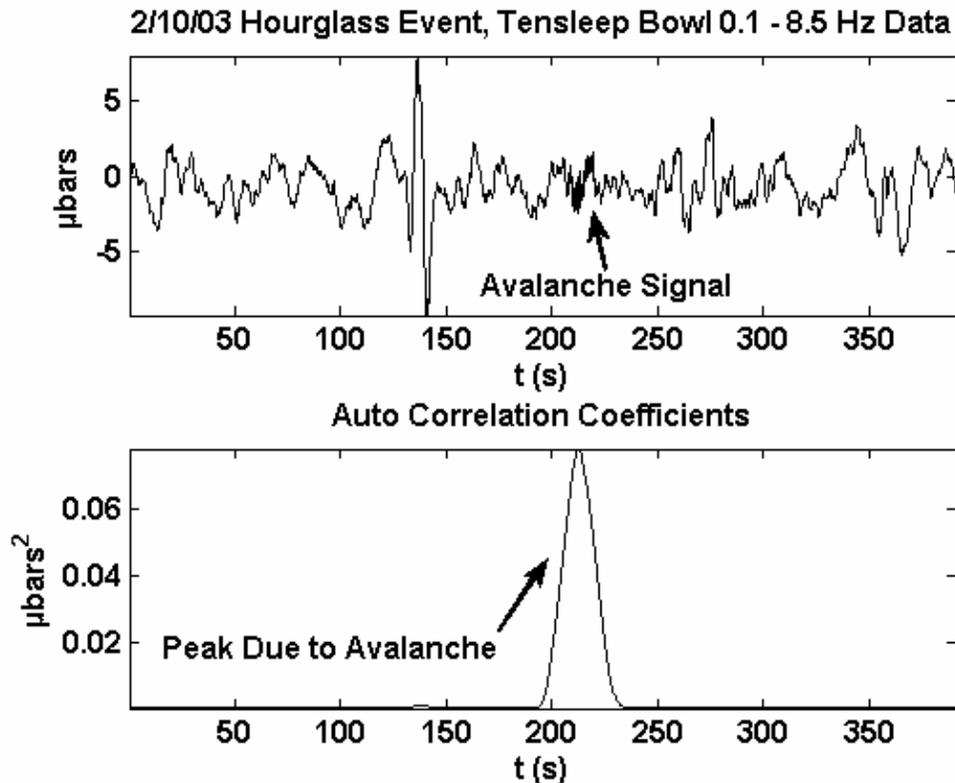
Figure 3. Class 2 Avalanche Signal and Low Wind Noise
