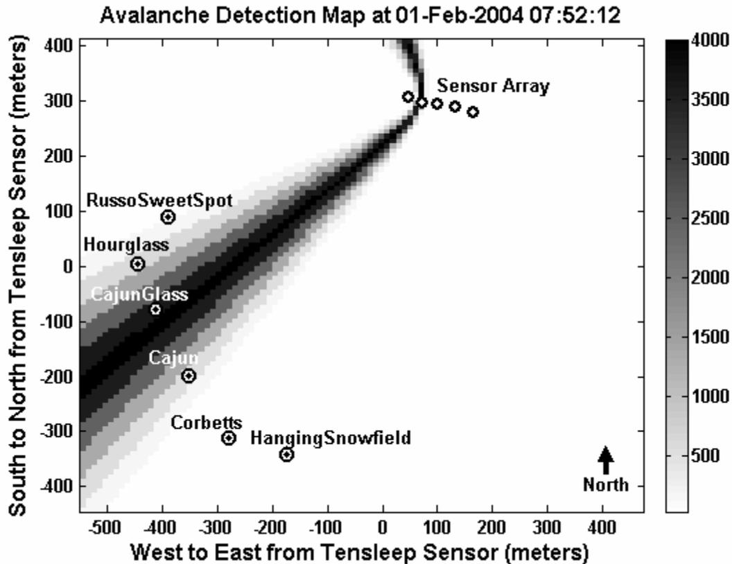
Figure 11. Sensor Array 2/1/04 CajunGlass Identification and Localization
