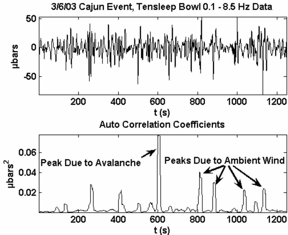
Figure 4. Class 2 Avalanche Signal and High Wind Noise
