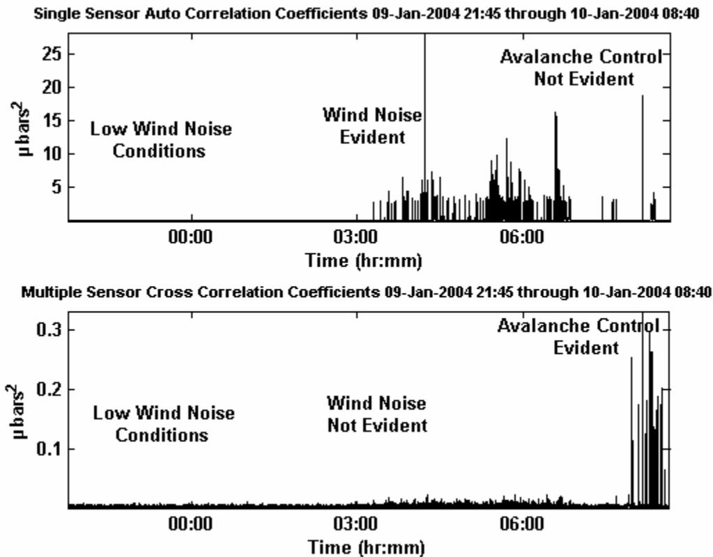
Figure 10. Single vs Six Sensor Signal Identification
