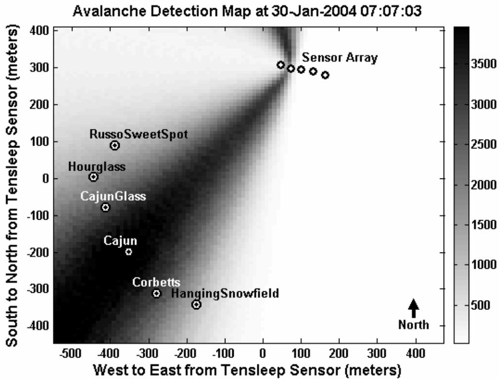
Figure 13. Sensor Array 1/30/04 Cajun Semblance Identification and Localization
