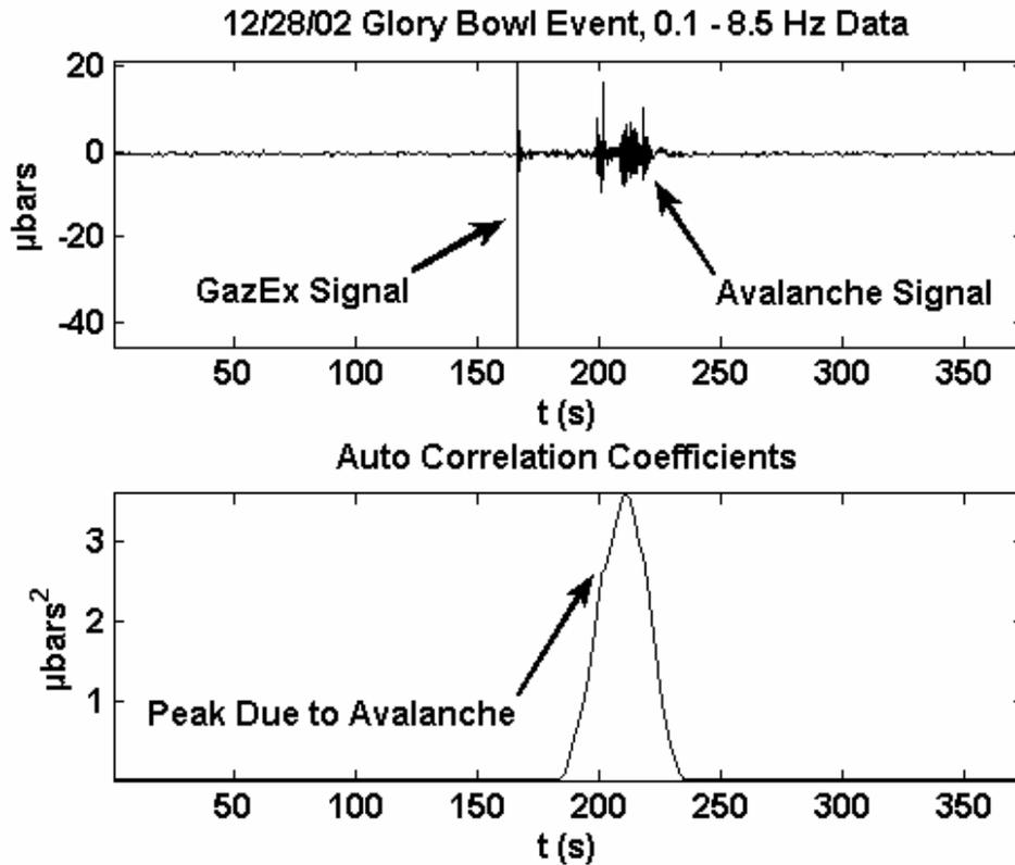
Figure 2. Class 3 Avalanche Signal and Low Wind Noise
