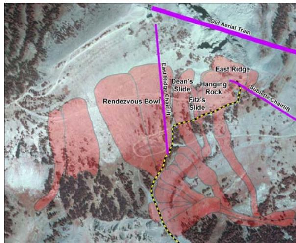
Figure 3: Outline of the extent of Class V size (relative to the path) avalanches that affect the route from the Sublette to East Ridge Lifts.
